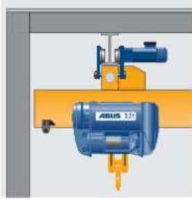
Standard main girder connection configuration – Version 1 (variable cantilever for minimum side approach dimension)
