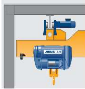
Standard main girder connection configuration Version 1, "angled" (variable overhang for minimum side approach dimension)
